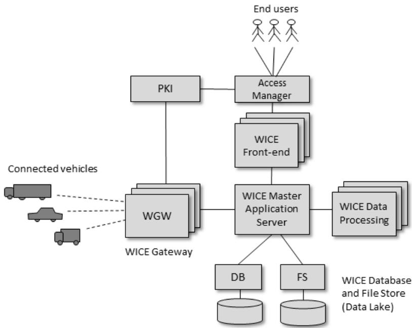
**Figure 2: High level architecture of the WICE back-end infrastructure**
